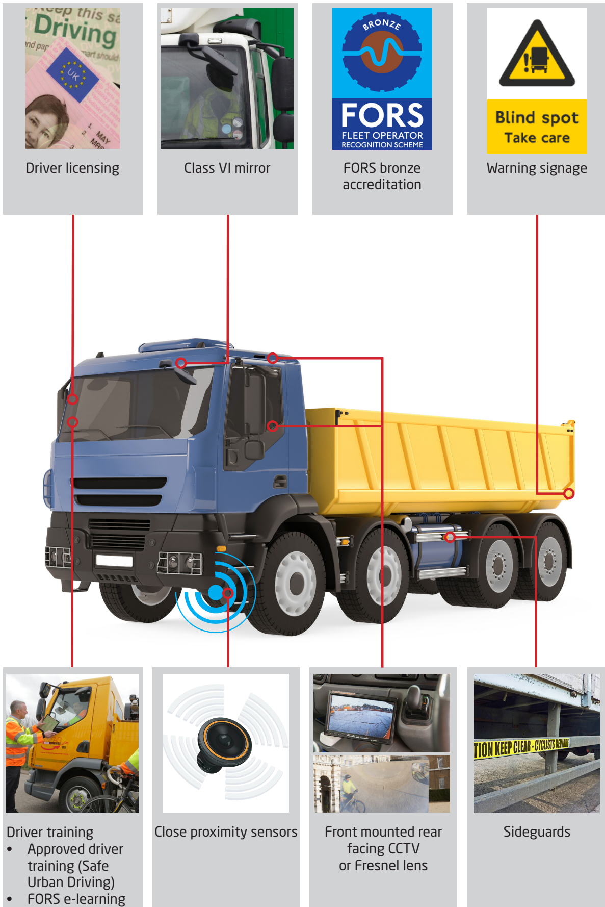
Figure 20 – WRRR requirements for vehicles above 3.5 tonnes
