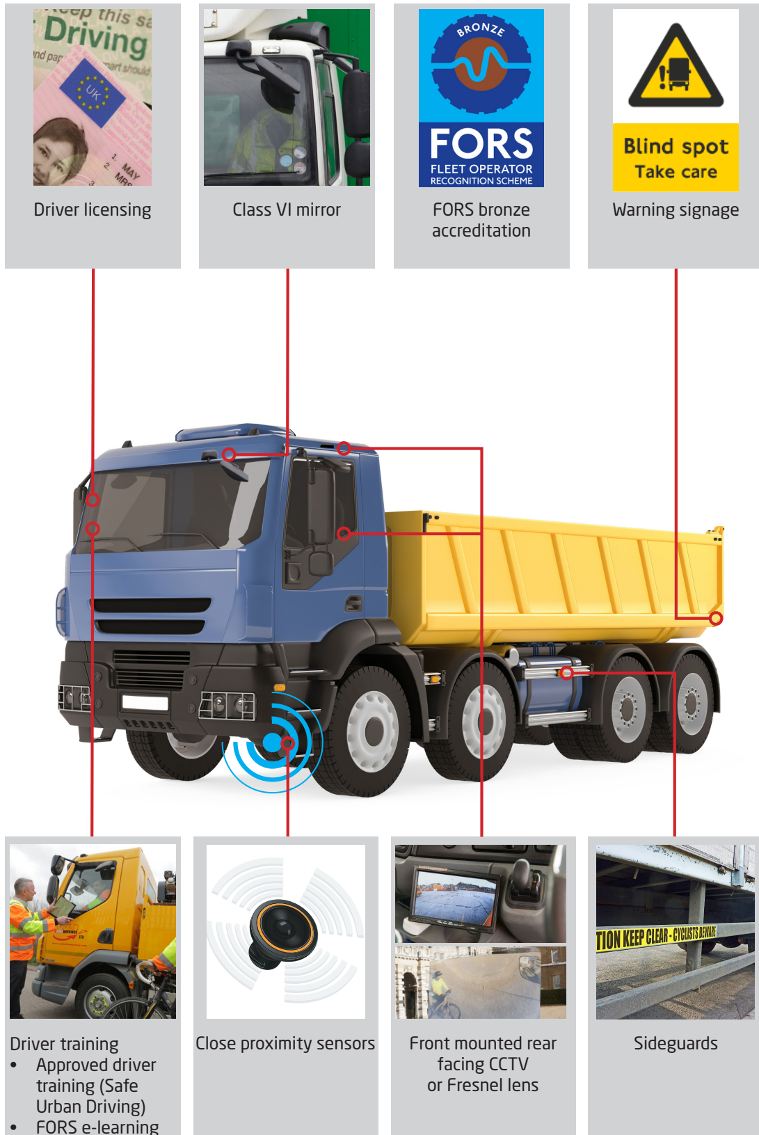
Figure 2 – WRRR requirements for vehicles above 3.5 tonnes
