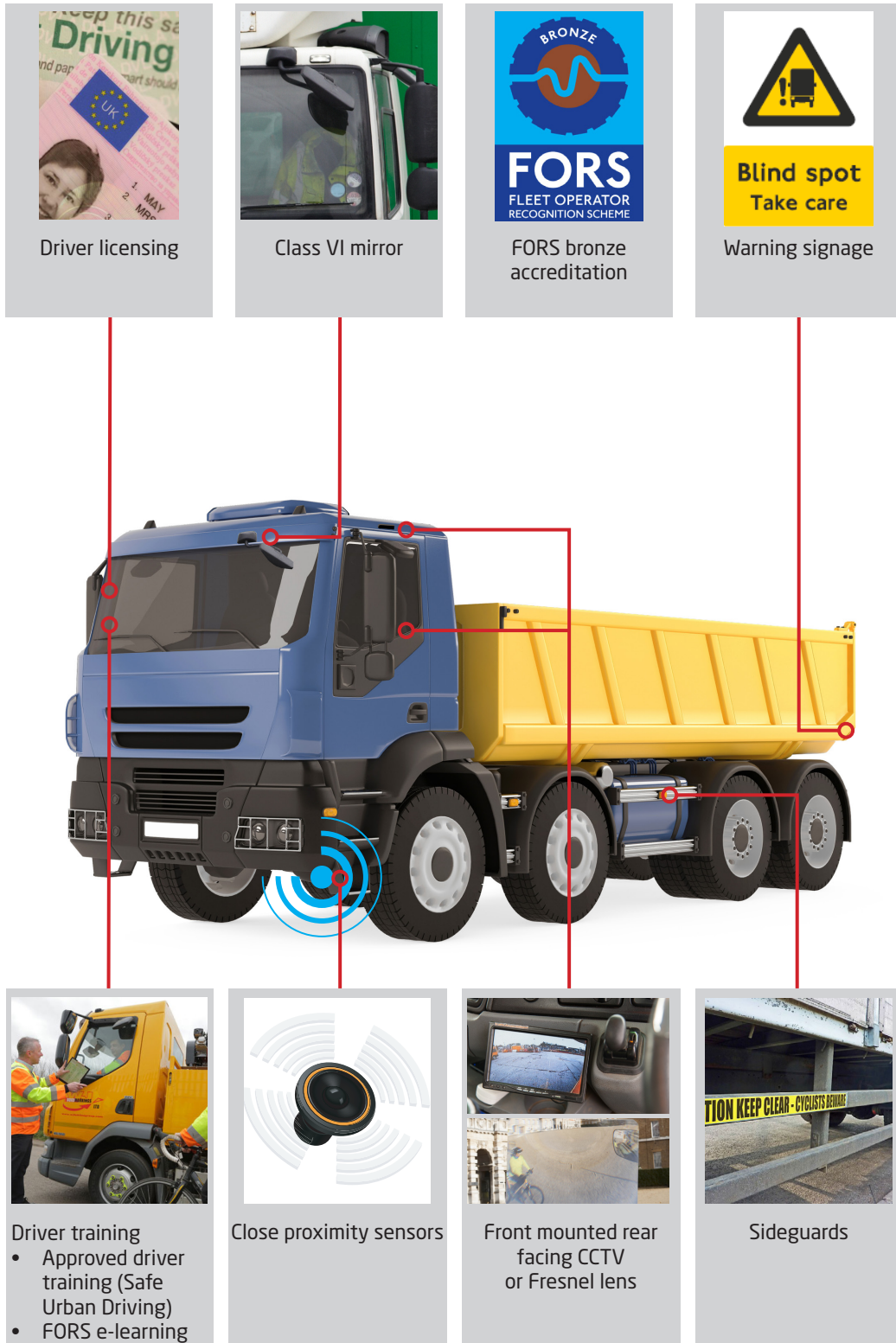
Figure 14 – WRRR requirements for vehicles above 3.5 tonnes
