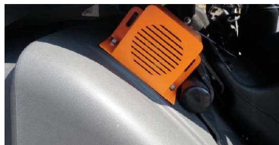
Figure 6: Audible warning system for left-turning
