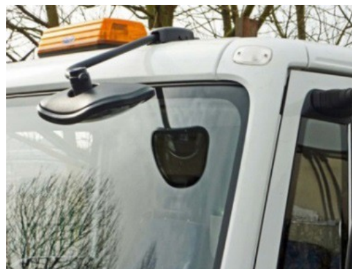
Figure 5: Class VI mirrors
