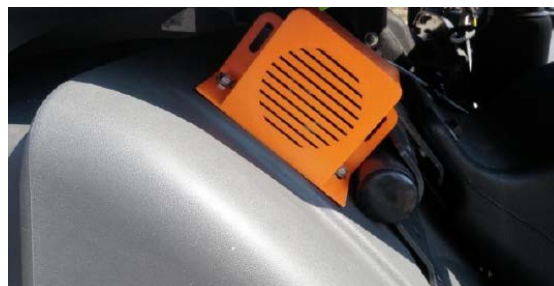
Figure 6: Vehicle manoeuvring warning for left-turning
