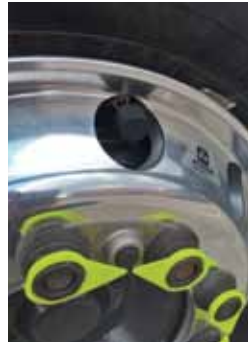
Wheelnut flags provide a valuable warning if a nut is on the move
