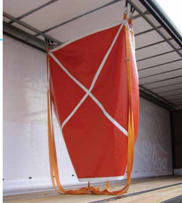
ABOVE: a 'kite' can be used to restrain loads that do not reach the back of the trailer
