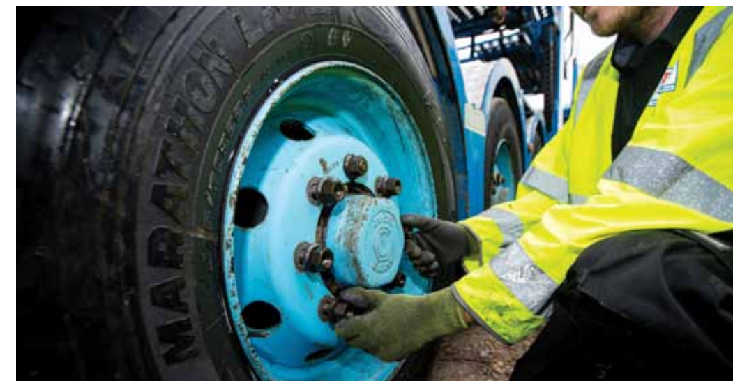
LEFT: nuts must be free-running on threads if a false torque is to be avoided
