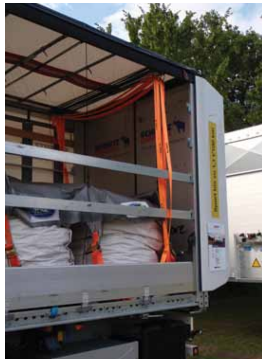
ABOVE: the German way – this Schmitz Cargobull trailer features toe boards, side laths and pull-down sheets
