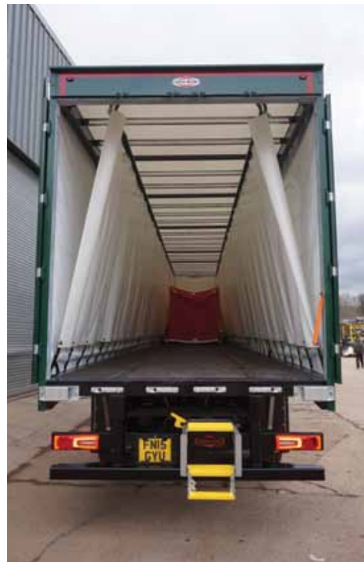
ABOVE: the German way – this Schmitz Cargobull trailer features toe boards, side laths and pull-down sheets
