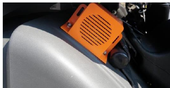
Figure 6: Vehicle manoeuvring warning for left-turning
