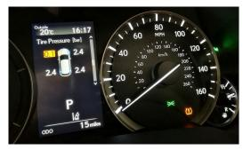
**Direct TPMS** – sensors within each tyre monitor actual pressure levels and report any anomalies directly to the driver via the dashboard
