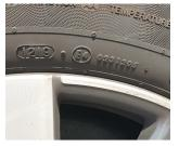
If you buy a retreaded tyre, make sure that it has the E-mark on it, which confirms that a tyre meets minimum EU or International (UNECE) standards in relation to its dimensions, load and speed rating. All motor vehicles tyres in the EU must be E-marked, whether new or retreaded.
