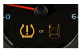
Indirect TPMS – the antilock braking system (ABS) uses wheel speed sensors to measure the rate of revolutions for each wheel. When the system detects that a wheel is spinning faster than expected due to it being under-inflated, it sends an alert to the driver
