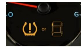
Indirect TPMS – the antilock braking system (ABS) uses wheel speed sensors to measure the rate of revolutions for each wheel. When the system detects that a wheel is spinning faster than expected due to it being under-inflated, it sends an alert to the driver
