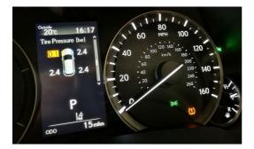
**Direct TPMS** – sensors within each tyre monitor actual pressure levels and report any anomalies directly to the driver via the dashboard
