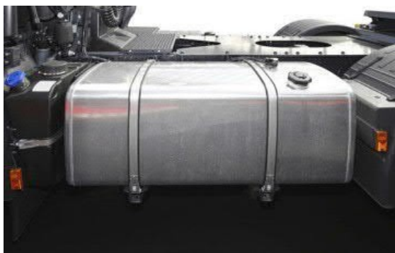
Figure 3: Example of fuel tank achieving the same objective as sideguards
