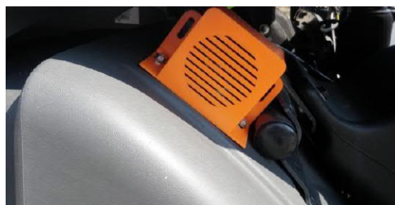
Figure 6: Vehicle manoeuvring warning for left-turning
