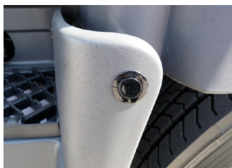
Figure 7: Close proximity sensor
