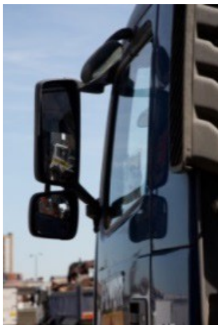
Figure 4: Class V mirrors
