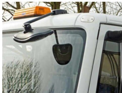
Figure 5: Class VI mirrors
