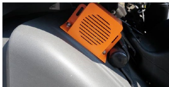
Figure 6: Vehicle manoeuvring warning for left-turning
