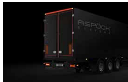
ABOVE – LED strip replaces top rear markers
