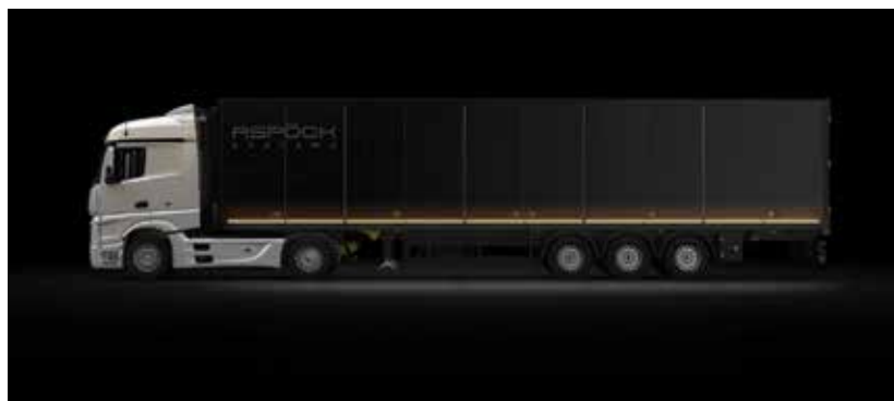
BELOW: LED strips replace individual side markers
