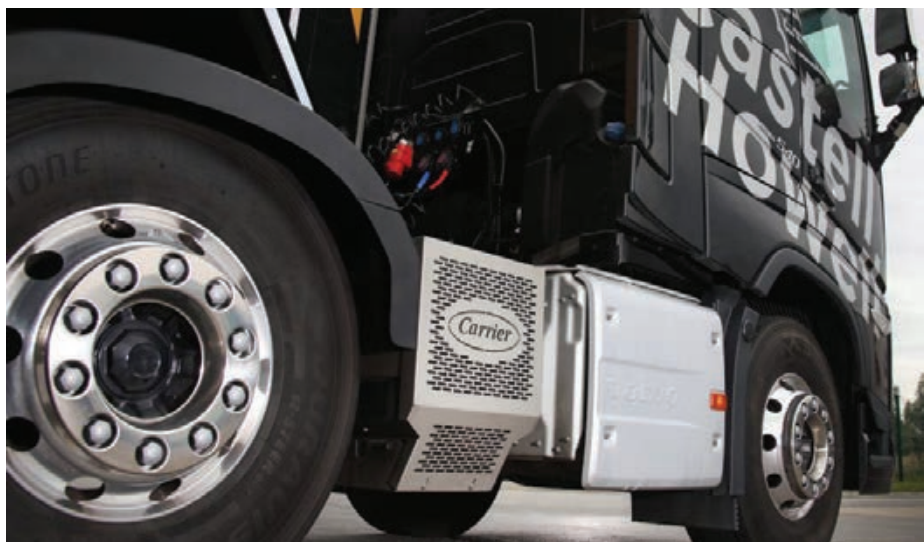
Left: Carrier Eco-Drive hydraulic generator runs off the truck's PTO
