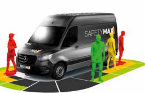
Left: Safetymax uses up to 16 ultrasonic sensors to provide drivers with a clear indication of obstacles around the vehicle
