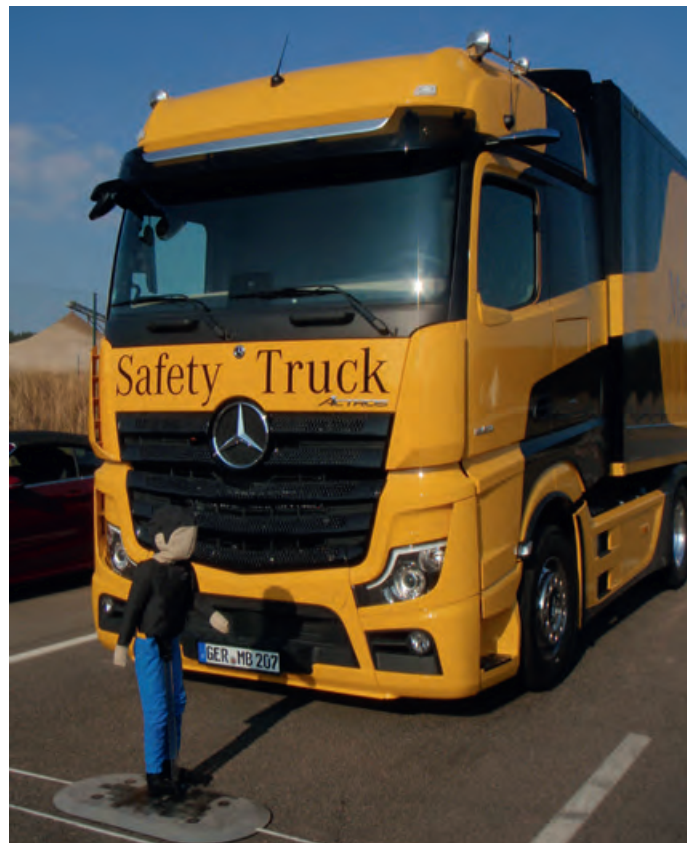
Above: A moving off information system protects vulnerable users in the blind spot to the front of the truck
